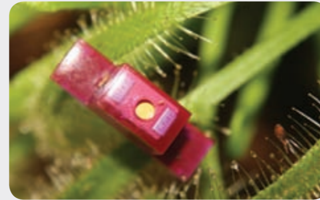
Integrated electronics: Sensor package made using additive technologies
