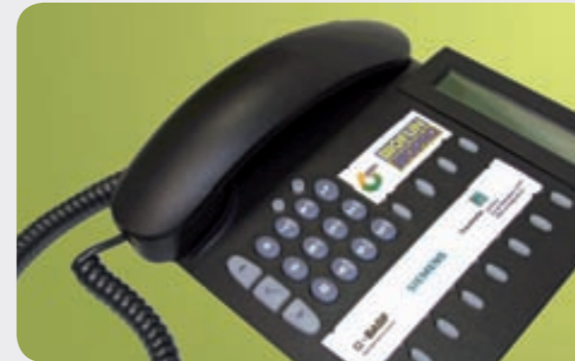
A functional project demonstrator showing the use of renewable resources ("bioplastics") in electronic applications
