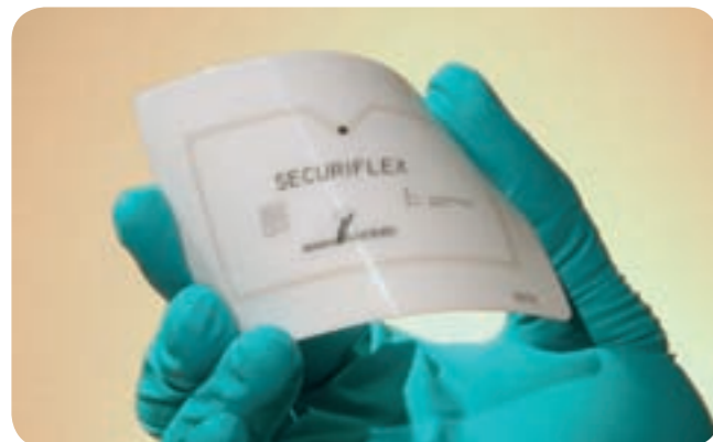
Extremely thin transponder for secure ID documents
