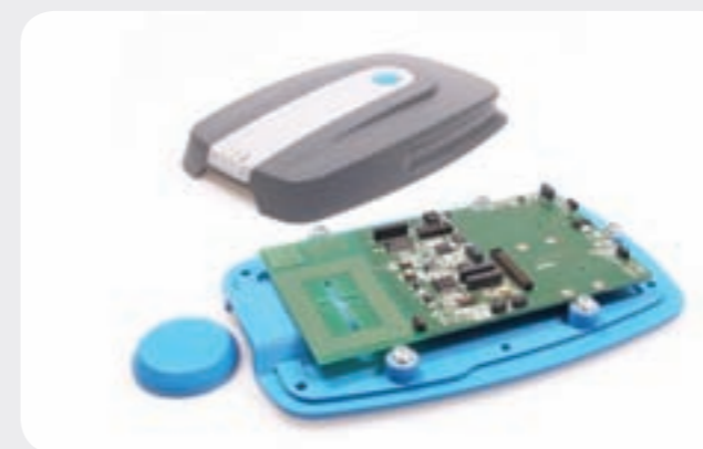
Multi sensor system with RFID interface, communication via GSM
